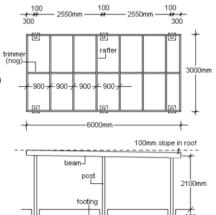
fer to these plans for any required measurements throughout the project.
