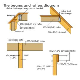
Cut the two end rafters 3000mm long with 45degree angle cuts each end and fix in place to the beams with 75mm jolthead galvanised nails and then with galvanised angle brackets, each bracket fixed with four M12 galvanised bolts, two through the beam and two through the rafter. (See diagram)
