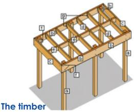
The timber for this project can be either sawn (rough sawn) or dressed (gauged, smooth finish). The timber measurements used in this project are for concept only and not to stock sizes. Please make allowances for the difference in timber thickness and width.
